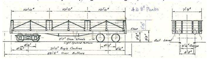
While the drawing shows the Queensland Railways version with diagonal bracing on side drop gates, the BTR HJ Class does not have these, much like the F Class wagons.
