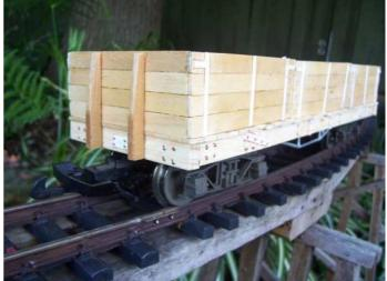
The flooring, frame, sole bars, buffer beams and planks are slit pine as are side gates and ends.
